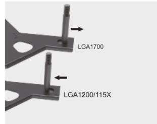
**[EN]** The Intel backplate is designed for LGA1700 and LGA1200/115X sockets. Push the screws to the outside for LGA1700. Push the screws to the inside for LGA1200/115X.
